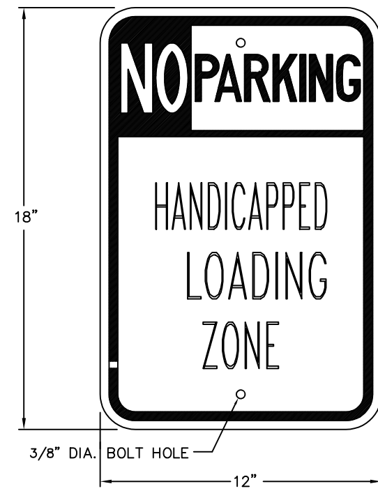
LETTERING, BORDER & SHADED AREAS-RED LETTERING ON LOWER PORTION OF SIGN TO BE CENTERED HORIZONTALLY WITHIN RED BORDER BACKGROUND-WHITE HANDICAPPED LOADING ZONE NOT TO SCALE
